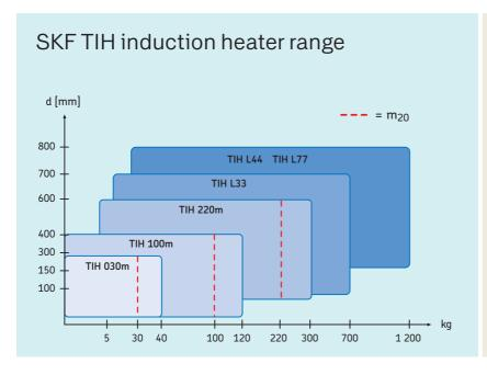
The comprehensive range of SKF induction heaters is suitable for most bearing heating applications. The chart gives general information on choosing an induction heater for bearing heating applications <sup>3)</sup>.
